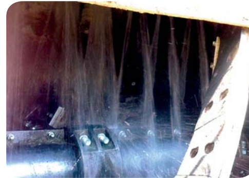
BASINÇLI MİKSER İÇİ OTOMATİK YIKAMA SİSTEMİ HIGH PRESSURE WASHING SYSTEM FOR MIXER.
