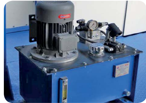
HİDROLİK ÜNİTE VE MANUEL KOL HYDRAULIC UNIT AND MANUAL ARM
