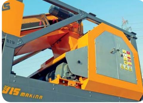
AÇILIR AGREGA GİRİŞ BOĞAZI OPENABLE AGGREGATE INLET.
